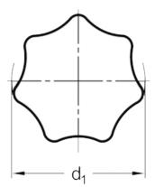
$\begin{array}{lll} d1 & = 32 \\ d2 & = M 6 \\ d3 & = 12 \\ h1 & = 20 \\ h2 & = 9 \\ t2 & = 10 \\ Weight in (g) = 54 \end{array}$
